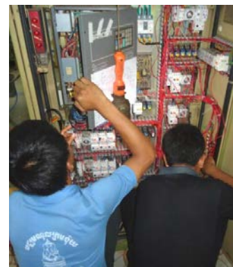
... or cigarette factory), a team of trainers under the supervision of Vannak, are working during this month of July on the reassembling of a cigarette packing machine, a second-hand purchase which has been lying idle for years in a warehouse. Without any documentation, (except a few indications in Chinese) the electrical circuits had to be read, the diagrams to be drawn, and the spare parts to be found, and the robots to be restarted... After a month work, the machine operates again in the production line... Congratulations to Vannak and his team... But this is not the end of it, there are still three other machines to reassemble.
