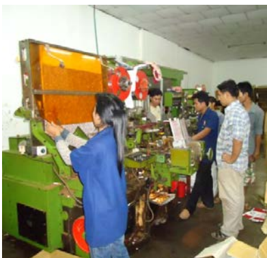
... or cigarette factory), a team of trainers under the supervision of Vannak, are working during this month of July on the reassembling of a cigarette packing machine, a second-hand purchase which has been lying idle for years in a warehouse. Without any documentation, (except a few indications in Chinese) the electrical circuits had to be read, the diagrams to be drawn, and the spare parts to be found, and the robots to be restarted... After a month work, the machine operates again in the production line... Congratulations to Vannak and his team... But this is not the end of it, there are still three other machines to reassemble.
