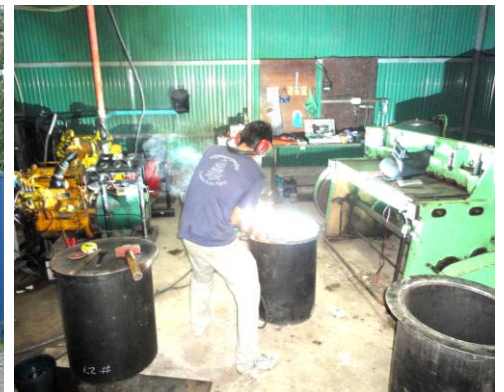
CKN Workshop at Phnom Penh Thmey . Building gasifiers and mechanics
