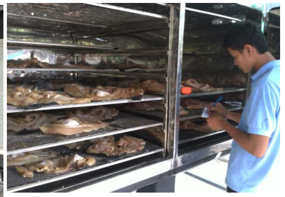
The Solar dryer at krakor starts working, producing 30 Kg/chamber of dried clean fishes every 25 hours.
