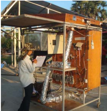
Sokpheap, a CKN teacher, experimenting her control electronic system in a small drying model
