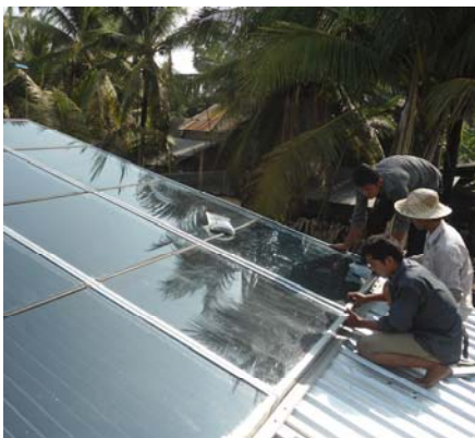
The Solar dryer at krakor starts working, producing 30 Kg/chamber of dried clean fishes every 25 hours.
