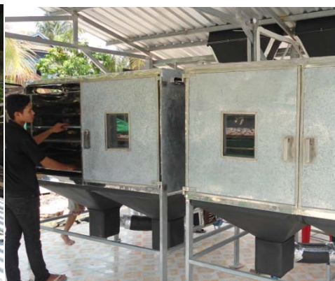
The Solar dryer at krakor starts working, producing 30 Kg/chamber of dried clean fishes every 25 hours.
