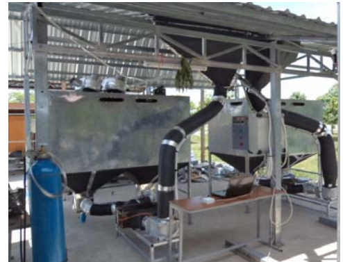
Building at CKN campus the solar dryer to be installed at Krakor (in Pursat province)
